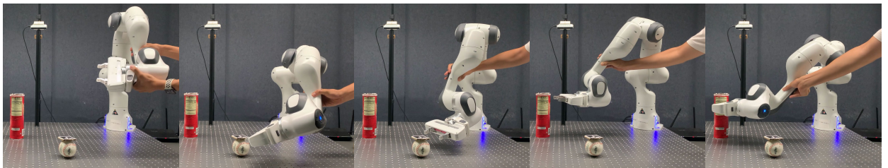
Figure 19: Shared control with virtual guides for the collaborative grasping of different objects.
